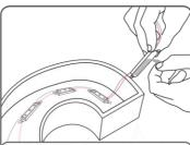
Using LED placement from step 1. remove tapes on the backside and stick LED modules into place.
