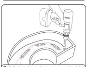
Orill the holes at the bottom or side of the letters for the wire connection to DC power supplies and grommet the hole for supply wire
