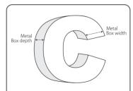
• Noting metal box depth, width and face material, use layout guidelines and power supply capacity charts on page 2 to determine spacing and quantity of LEDs.
