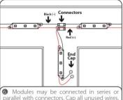
Modules may be connected in series or parallel with connectors. Cap all unused wires. The strand of modules should not be looped to reate a closed circuit
