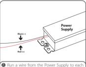
Run a wire from the Power Supply to each channel letter and connect to the first LED module on the strip. Must be used with 12 V BaltLED Power Supplies.
