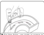
For firm fixing, use rivets or screws to secure the LED strip within the channel
