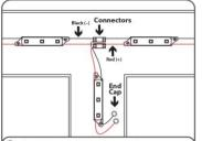
6 Modules may be connected in series or parallel with connectors. Cap all unused wires. The strand of modules should not be looped to create a closed circuit.
