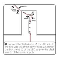
! 30 pcs - max number of modules in one chain when the power supplied from single end. ! String end voltage can't be less than 11V, do not exceed specified module string length
