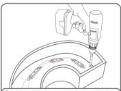
Orill the holes at the bottom or side of the letters for the wire connection to DC power supplies and grommet the hole for supply wire access.
